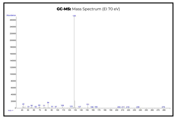
**Confirmation Using Drug Standard:** Reference material (Batch: 0500950-12) was purchased from Cayman Chemical (Ann Arbor, MI, USA). The analyte was confirmed to be MMMP based on retention time (sample: 6.40 min vs. standard: 6.39 min) and mass spectral data comparisons.
