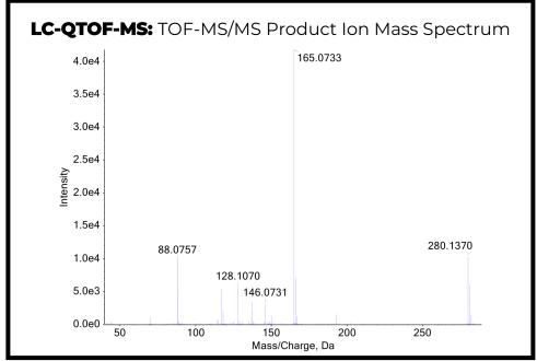
**Confirmation Using Drug Standard:** Reference material (Batch: 0500950-12) was purchased from Cayman Chemical (Ann Arbor, MI, USA). The analyte was confirmed to be MMMP based on retention time (sample: 6.58 min vs. standard: 6.47 min) and mass spectral data comparisons.
